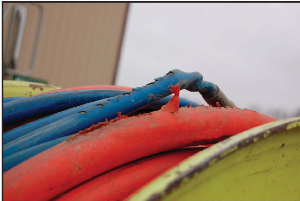
Above: An example of damaged hose which should be replaced.
