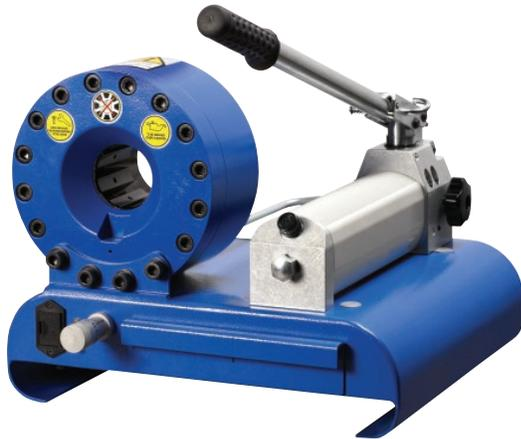
**Description:** Looking for a reliable crimping tool that won't take up a lot of space? With its small footprint the KC1-H47PM is a perfect fit for crowded shops. Its small size also makes it suitable for quick trips into the field.
