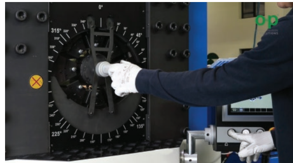
Tool held in place by built-in locking posts inserted into the crimper on smaller and larger sized crimpers.
