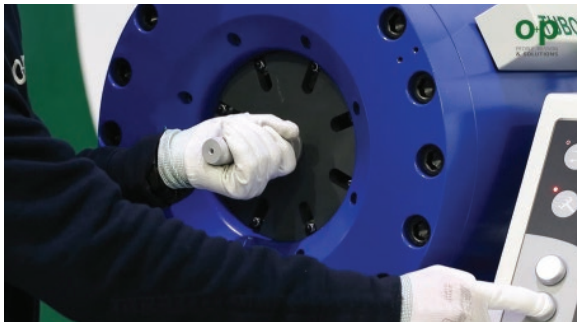
Master dies are guided through built-in channels on the tool on mid-sized crimpers.
