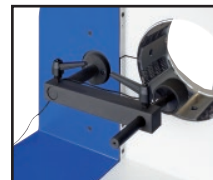
Back Limit Switch
