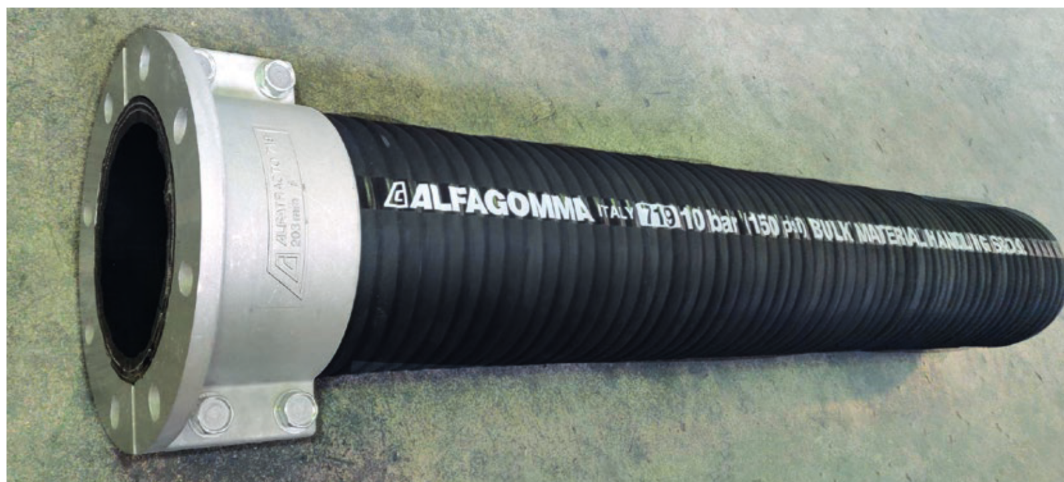
4 Place the two half shells onto the hose and tighten the side flange bolts. The corrugation inside the muff coupling must align exactly with the corrugation of the hose cover
